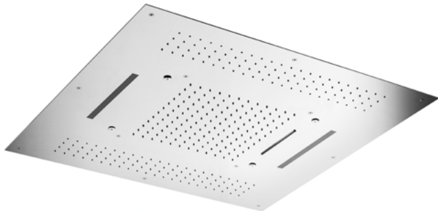
Spa built in chromotherapy multifunction shower head • AISI 304 stainless steel • 4 function shower • LED lighting • Water-resistant lighting remote control • Recommended thermostatic mixer: 780240200 • Antiscale • 950x950 mm
