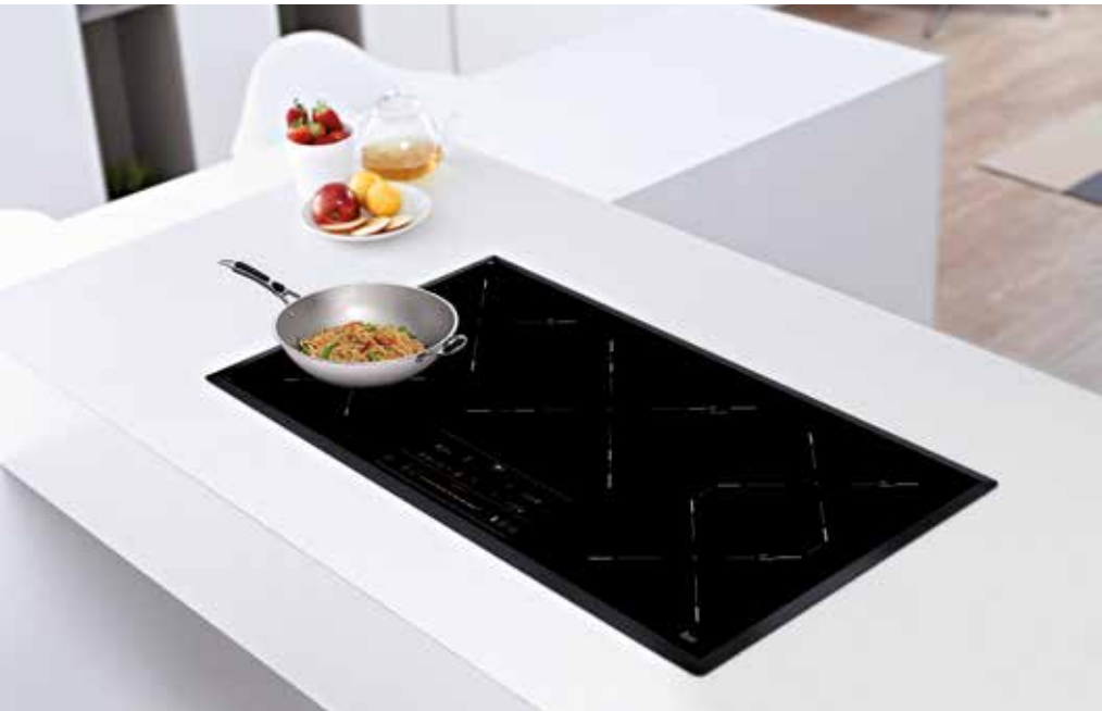
Induction technology An electromagnet located beneath the glass surface creates a powerful magnetic field which fits the size and shape of the cookware and heats only its base while adjacent areas remain cold. Up to 90% of the energy consumed is transferred to the pot being used.
