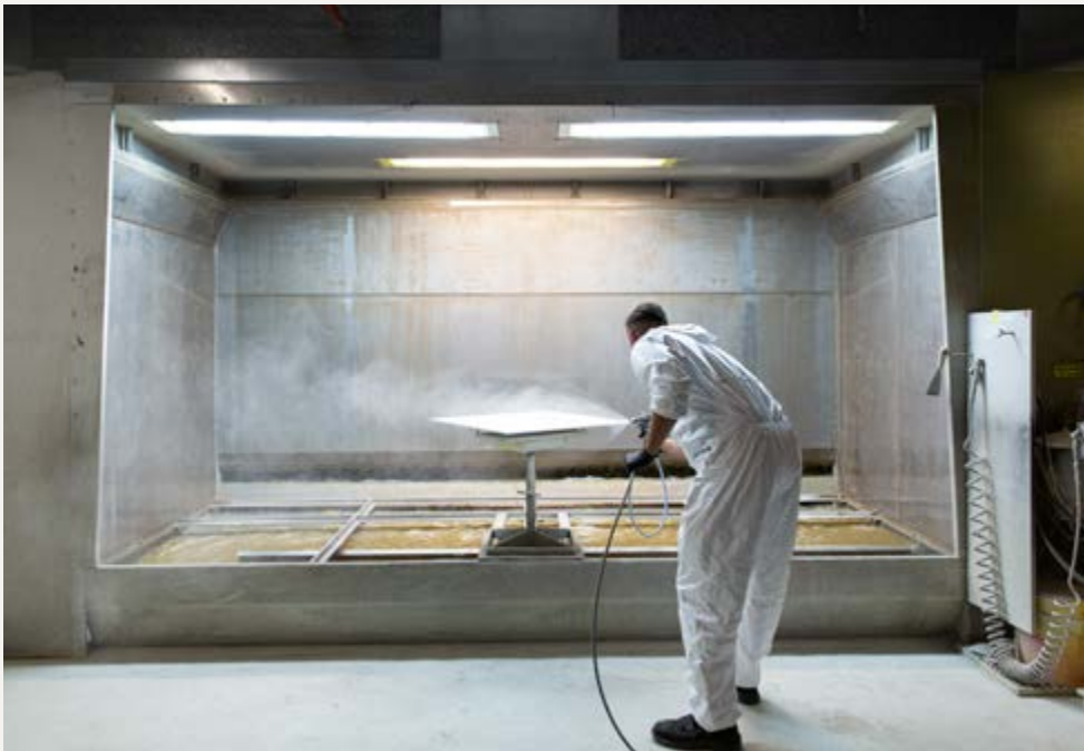
Following precision digital cutting, which is accurate to a tenth of a millimetre, the lacquer finish is applied. Each front panel is processed from all sides. The paint must be applied accurately right into the groove on the side to prevent subsequent moisture penetration.
