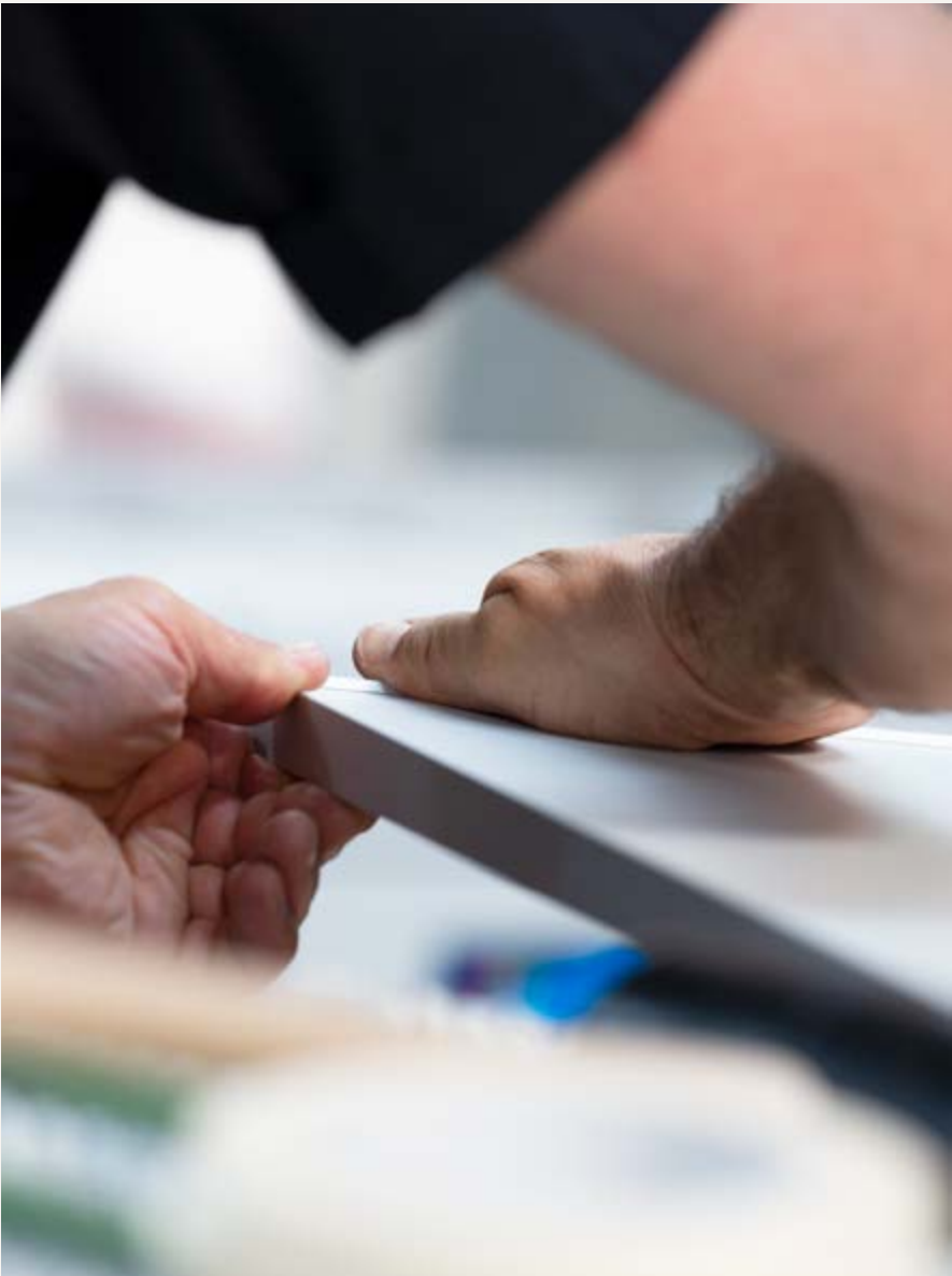
Special skill is also required to mount the frame. The fine strips are individually set in the circumferential groove before each mitred corner is manually adjusted.
