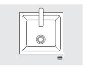
Mixer behind the sink, control element mounted on the front of the kitchen worktop
