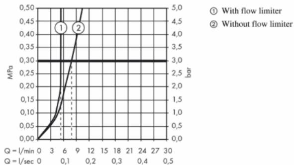
The consumption was measured in combination with the appropriate fittings (thermostat/mixer/in-wall valve) to reflect actual application in practice.
