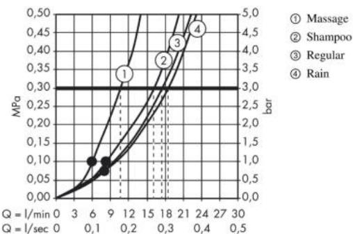
The consumption was measured in combination with the appropriate fittings (thermostata/mixer/in-wall valve) to reflect actual application in practice.
