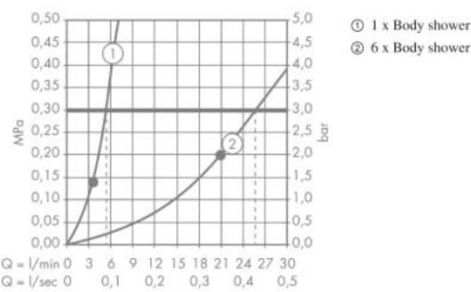
The consumption was measured in combination with the appropriate fittings (thermostat/mixer/in-wall valve) to reflect actual application in practice.
