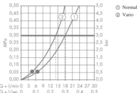
The consumption was measured in combination with the appropriate fittings (thermostat/mixer/in-wall valve) to reflect actual application in practice.
