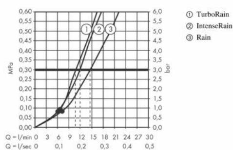
The consumption was measured in combination with the appropriate fittings (thermostatic/mixer/in-wall valve) to reflect actual application in practice.
