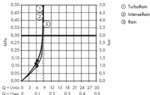
The consumption was measured in combination with the appropriate fittings (thermostat/mixer/in-wall valve) to reflect actual application in practice.
