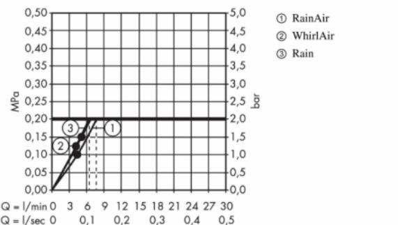
The consumption was measured in combination with the appropriate fittings (thermostat/mixer/in-wall valve) to reflect actual application in practice.
