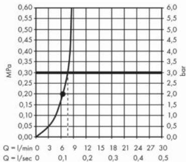
The consumption was measured in combination with the appropriate fittings (thermostat/mixer/in-wall valve) to reflect actual application in practice.
