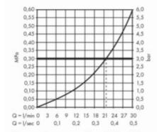
The consumption was measured in combination with the appropriate fittings (thermostat/mixen in-wall valve) to reflect actual application in practice.
