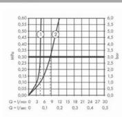
① With flow limiter ② Without flow limiter
