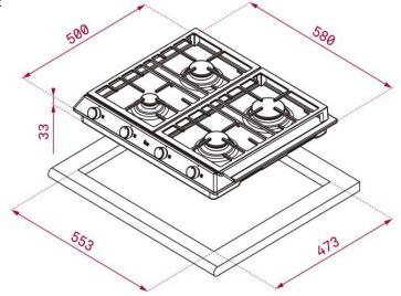
ATTENTION: Cut hole must be with round corners in order to avoid cracking on the counter-top.
