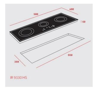
ATTENTION: Cut hole must be with round corners in order to avoid cracking on the counter-top.
