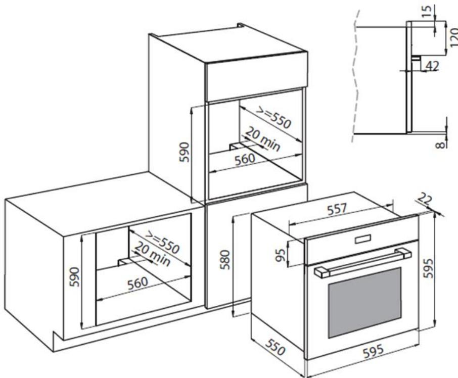
**Minimum 200mm<sup>2</sup> ventilation space at back of housing unit must be required.**
