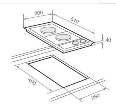
ATTENTION: Cut hole must be with round corners in order to avoid cracking on the counter-top.
