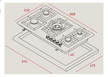
**ATTENTION:** Cut hole must be with round corners in order to avoid cracking on the counter-top.
