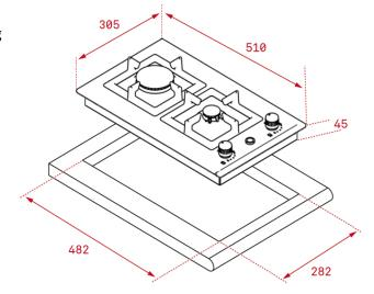
ATTENTION: Cut hole must be with round corners in order to avoid cracking on the counter-top.
