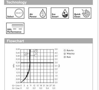
The consumption was measured in combination with the appropriate fittings (thermostat/mixer/
